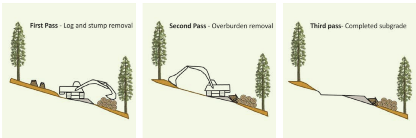
FIGURE 132. Each step of the way, the excavator clears vegetation and grubs the slope surface in front of it before it excavates and extends the road bench. Excavated soil from the new segment of road bench is placed and compacted on the new road bench and on the grubbed slope below the new segment. Cleared vegetation placed along the base of the future fill slope helps contain erosion from the exposed fill materials until they stabilize and revegetate (Modified from: BCMF, 1991).
